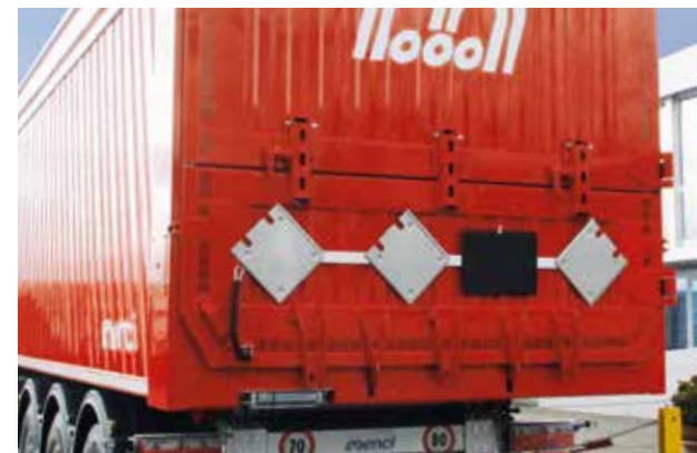
Door G with rod transport hatch
